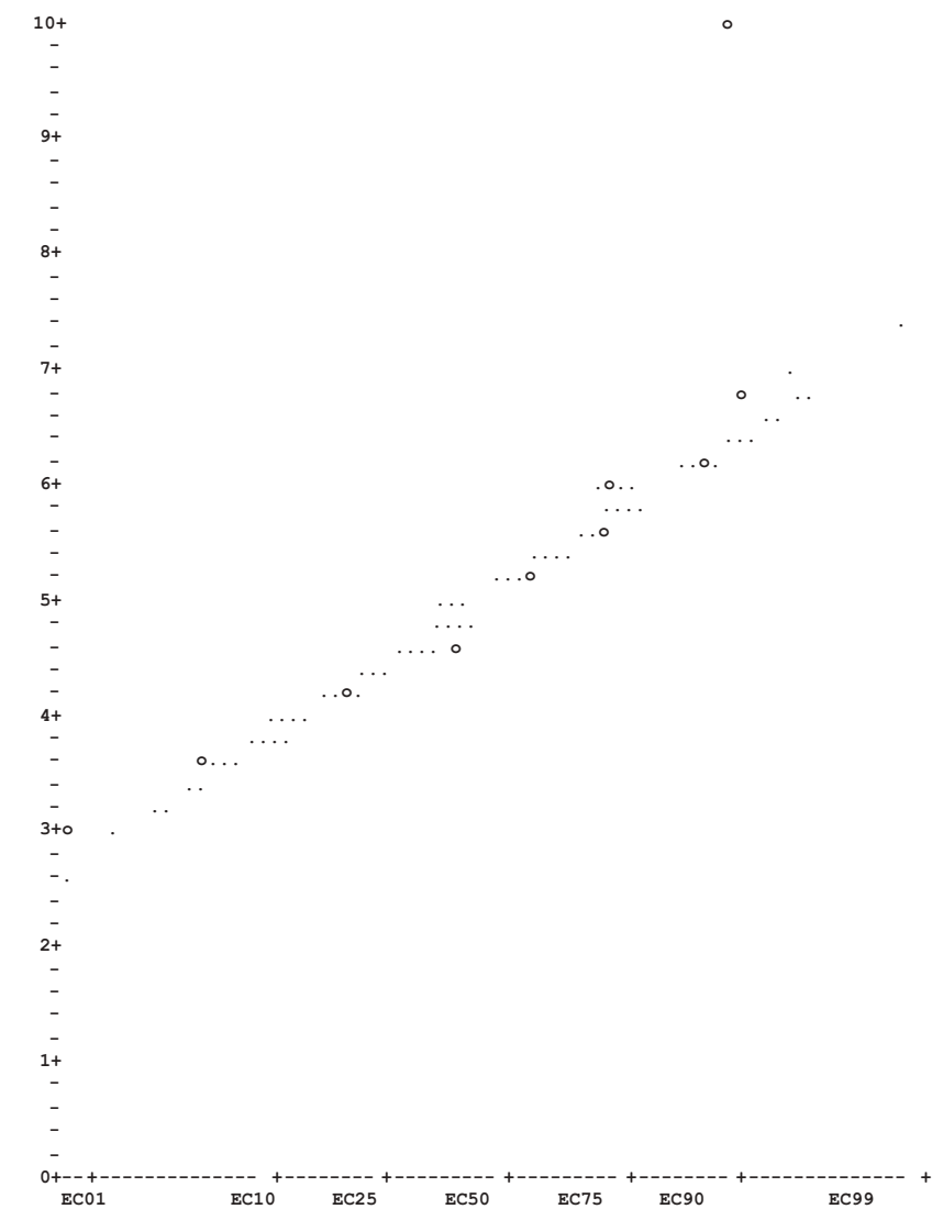
Fig1. Plot of adjusted probits and predicted regression line for 96 h LC 50 Probit
